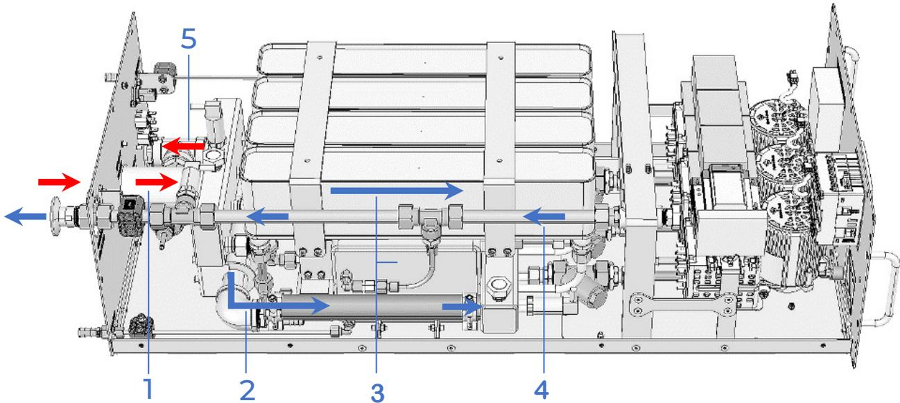
1. Heated **vapor refrigerant** flows from the servers towards the **condenser**.
